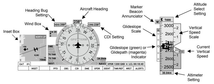
**INSET** - PRESS this Soft Key to view the Soft Keys which allow features to be displayed in the inset box (the box in the lower left corner of the PFD). They are:
