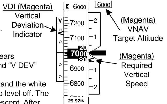
When the TOD point is reached, “ALT” changes to “VPTH” and the white “VPTH” changes to “ALTS” showing that 6000 ft is armed to level off. The Aircraft pitches down to achieve the programmed rate of descent. After the aircraft levels off at 6000 ft the green “VPTH” changes to “ALT” and the VDI, rate of descent chevron and the Target Altitude box all disappear.
